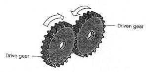
The drive gear is the gear that is turned by an outside effort, for instance your hand or an engine. Any gear that is turned by another gear is called a driven gear. The drive gear provides the input force and the driven gear delivers the output force.
